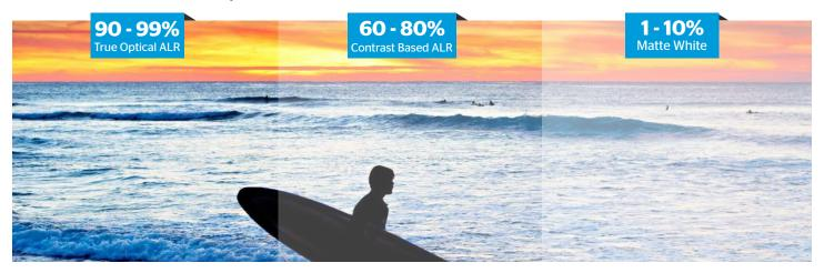
Side by side illustration of Ambient Light Rejection surfaces; True Optical ALR screens reject the highest percentage of ambient light, providing the best image contrast, color saturation and dynamic range.
