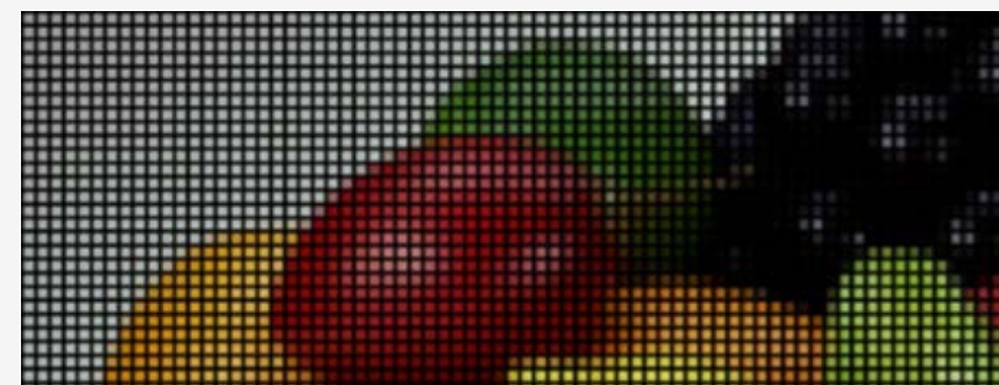
Wide inter-pixel gaps can make it seem as though you're looking at the image through a screen door. Hence the name "screen-door effect."
